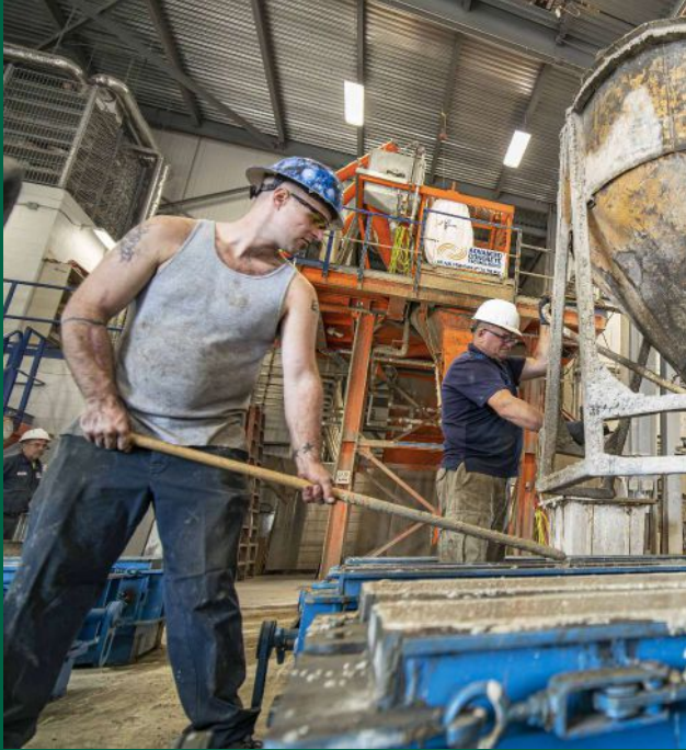
Team member Devon Cane (left) finishes a roadside curb from a fresh batch of self-consolidating concrete. The high spread mix design requires little or no vibration. Richard Swann checks production batch tickets for a Department of Transportation job on the ACT/Wiggert WGS Control.
