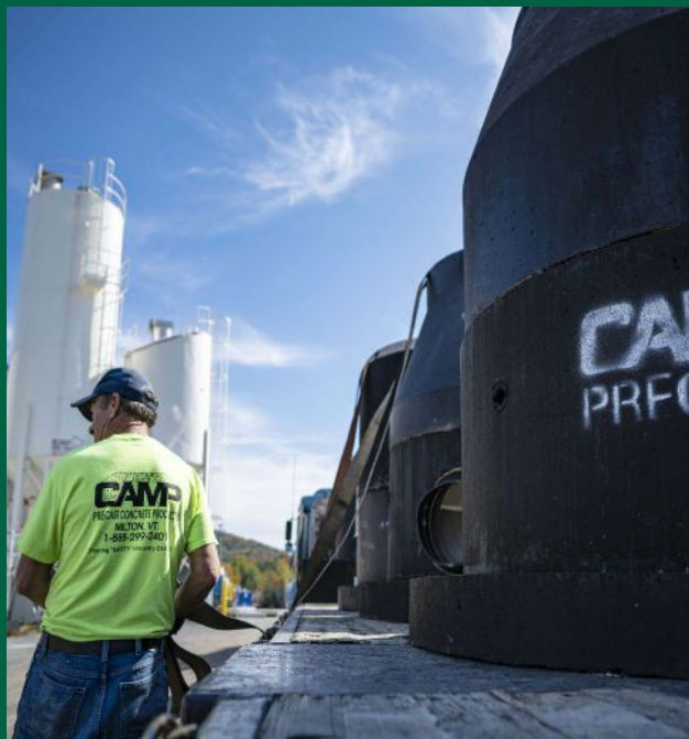
Dennis Alderman secures a load of Camp Precast coated manholes for delivery, while Ethan Camp caps a quality control inspection by stenciling the NPCA certified plant logo onto an electrical vault ready for shipment.
