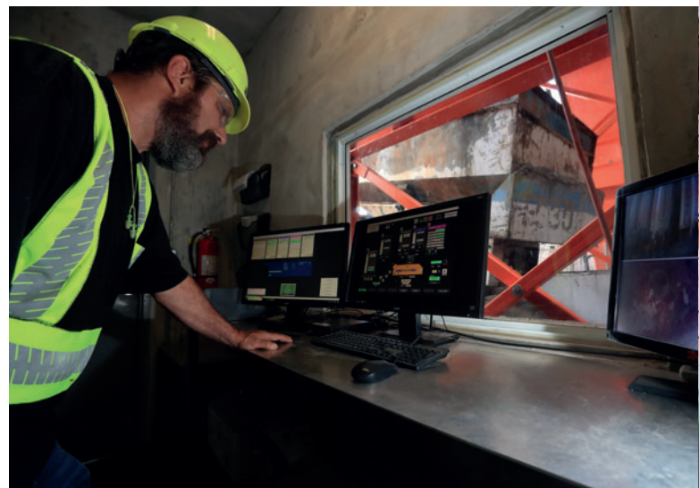
Fig 8: Plant manager Tom Garred checks on production and daily statistic using the ACT/Wiggert WCS control system while a Tucker reloads outside the control room window.
