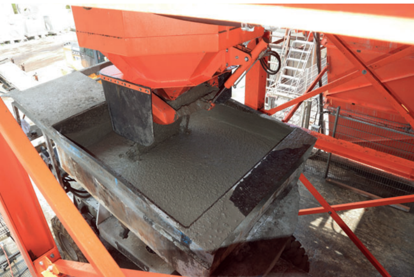
Fig 6: The new ACT/Wiggert batching system, with integrated 3 CY concrete holding hopper, can load a 6 CY capacity Tuckerbuilt concrete transport vehicle in under a minute.
