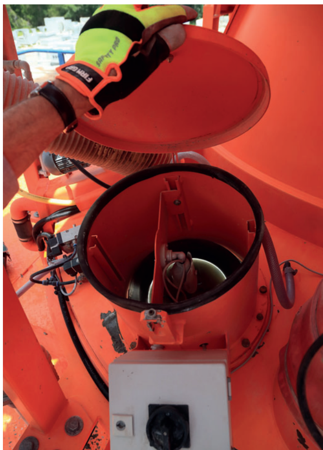
Fig 7: A video camera with light allows operator to view the concrete mix inside mixer remotely from the control room.
