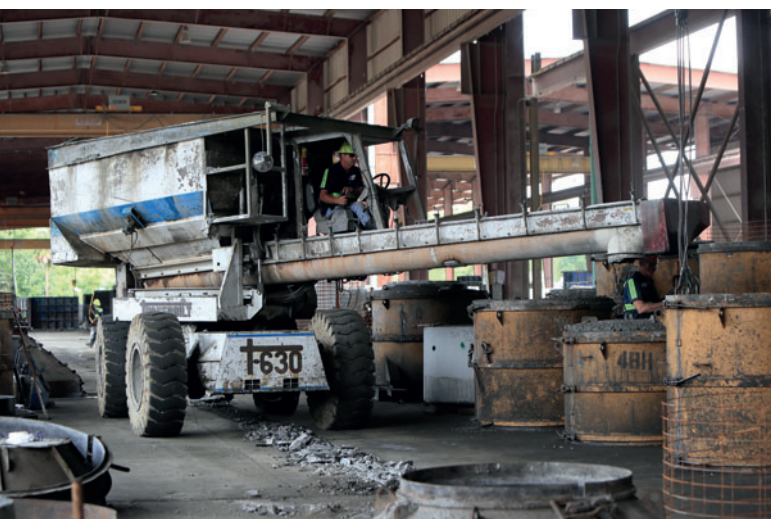
Fig 14: A 6-CY capacity Tuckerbilt concrete transport vehicle fills forms on the production floor at Forterra's Deland, Florida wet cast plant.
