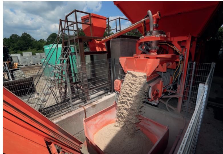
Fig 4: Integrated automatic Xypex admixture metering system accurately dispenses correct dosage of admixture powder.
