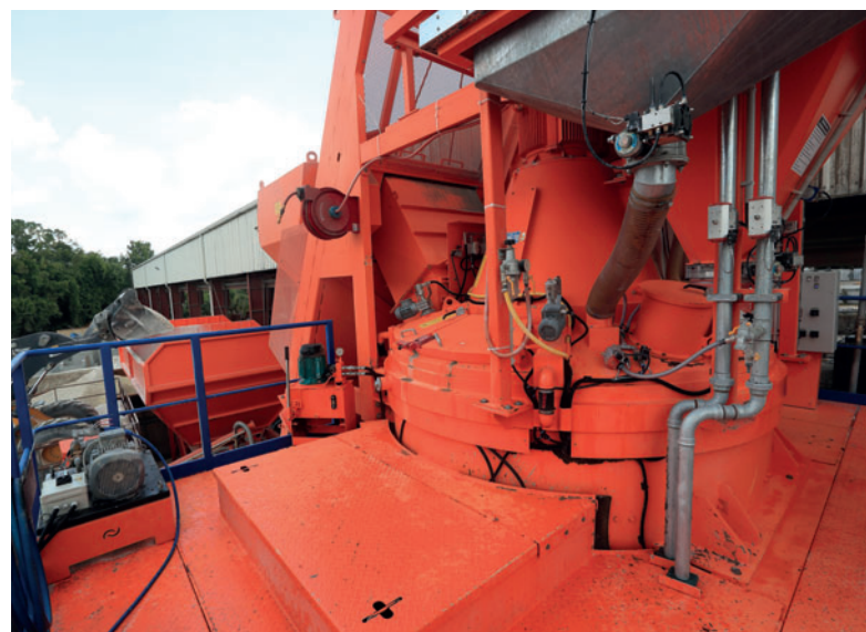
Fig 5: Even after 6 months of continuous use, the HPGM 3450 (3 CY) planetary mixer still looks like new thanks to good housekeeping practices and an automatic mixer cleaning system.
