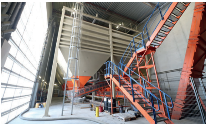
Fig. 14: The indoor heated 8-compartment aggregate storage systems used with both of Eagle Builders' ACT/Wiggert batching systems can each hold up to 1,600 tons of sand and stone to enable continuous operations even in the harshest weather.
