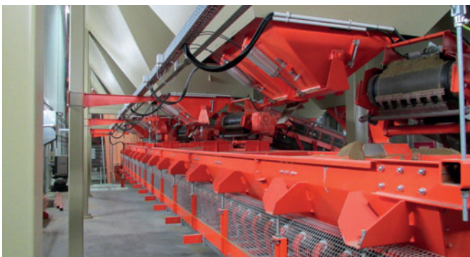
Fig. 15: Eagle Builders' custom-made aggregate bins are equipped with ACT dual-gate batching cones for precision coarse/fine batching. The aggregates are deposited onto an ACT weigh belt and then charged into a skip hoist on the ACT WicoMix 4500-WCS batch plant.
