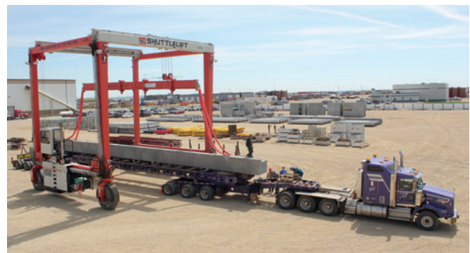
Fig. 16: One of three outdoor rubber-tired gantry cranes from Shuttlelift is used to load a precast beam onto a special trailer for delivery to a job site in western Canada.
