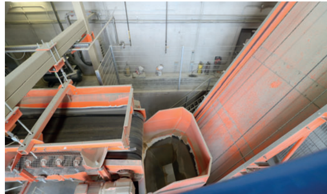
Fig. 14: The indoor heated 8-compartment aggregate storage systems used with both of Eagle Builders' ACT/Wiggert batching systems can each hold up to 1,600 tons of sand and stone to enable continuous operations even in the harshest weather.
