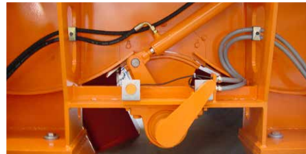
- DWM - Concrete discharge. ▲
