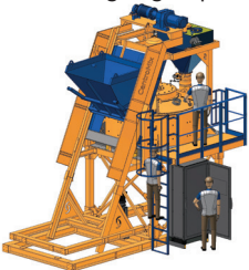
Diagram 1. Mixer platform with weighing skip
