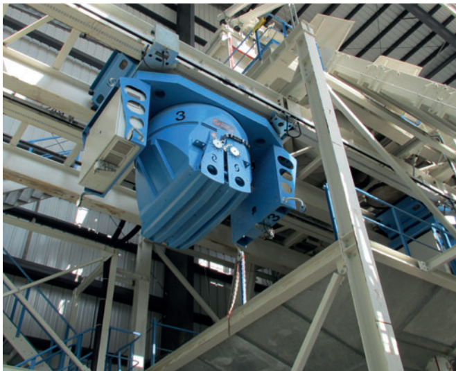
Fig. 7: One of four flying buckets is poised below its mixer discharge gate awaiting the next batch of fresh dry cast mix.
