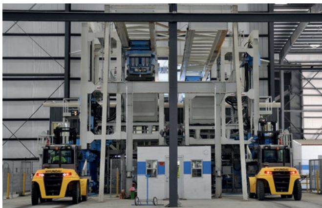
Fig. 11: The AmeriTex Conroe plant, completed in September 2016, features two Topwerk, Prinzing-Pfeiffer Radial Press packerhead style systems, including the RP 1225 for pipe 12" - 48" and RP 1625 for pipe 12" - 60" with variable lengths from 4' up to 8'.
