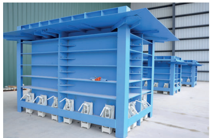
Fig. 15: Box culvert fabrication utilizes adjustable mold jack-ets and adjustable base pallets. The configuration equips AmeriTex with a wide range of capability, from variable box culverts, to large O-Ring joint pipes, arch or elliptical pipes.
