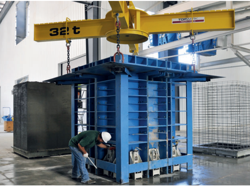
Fig. 16: An adjustable cross beam is used to move a box culvert form system into place over a reinforcing cage and pallet base in preparation for the move to the Variant production system.
