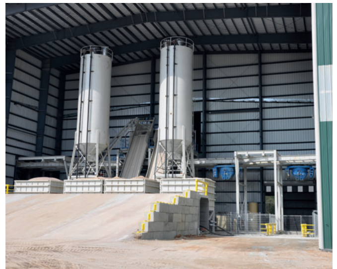
Fig. 8: Compact, modular design of the ACT/Wiggert MobilMat Mo 3450 batching system takes up very little space and is easily housed in a weather-tight structure at the AmeriTex Conroe plant.
