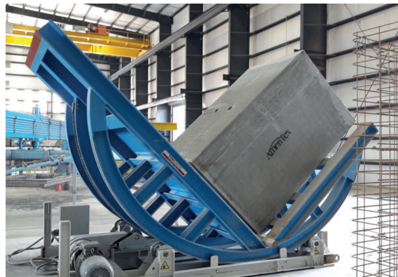
Fig. 18: A product tipping system from Topwerk can safely handle products weighing up to 24 tons. This system enables the Conroe plant to reorient products in preparation for transport to the storage yard. This system reduces or eliminates product damage associated with tipping and is safer than other tipping methods such as the use of a sand pit.
