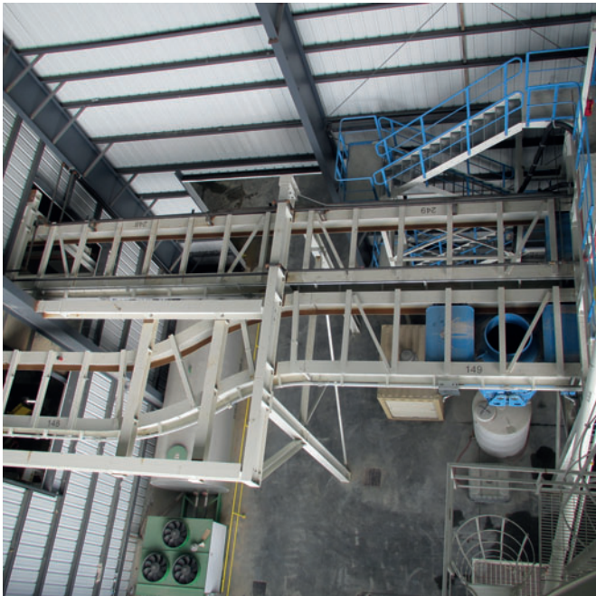
Fig. 9: A view from above the flying bucket track shows how the course can be configured to accommodate almost any system layout.
