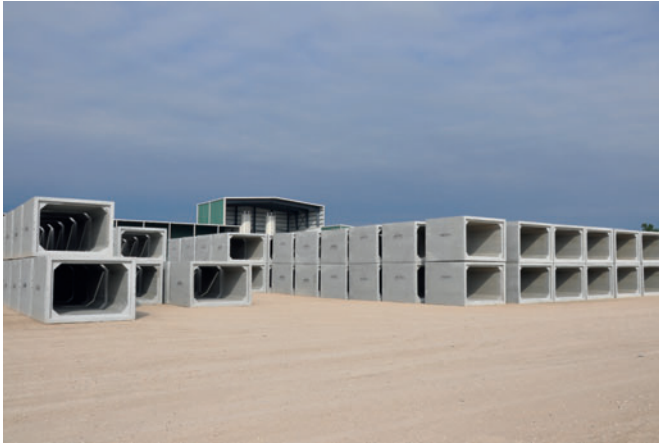
Fig. 3: Recently produced box culverts with variable lengths of 5' up to 8' are stacked in the storage yard awaiting delivery to various job sites.
