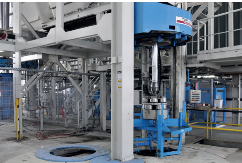
Fig. 17: The elements of the Topwerk, Prinzing-Pfeiffer Quick Change System are shown here. The new QCS system reduces pipe size change time from 90 minutes to 30 minutes or less, enabling multiple pipe sizes to be easily produced in a single shift.
