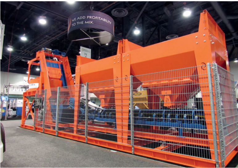
The new CentroMix plant introduced with 2 aggregate bins, accumulative weighing system & galvanized safety enclosure.
