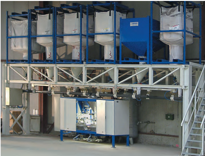
▲ COM 70-3 Granule metering system with three conveying vessels for 6 colors in 3 mixers with one electronic weigh hopper
