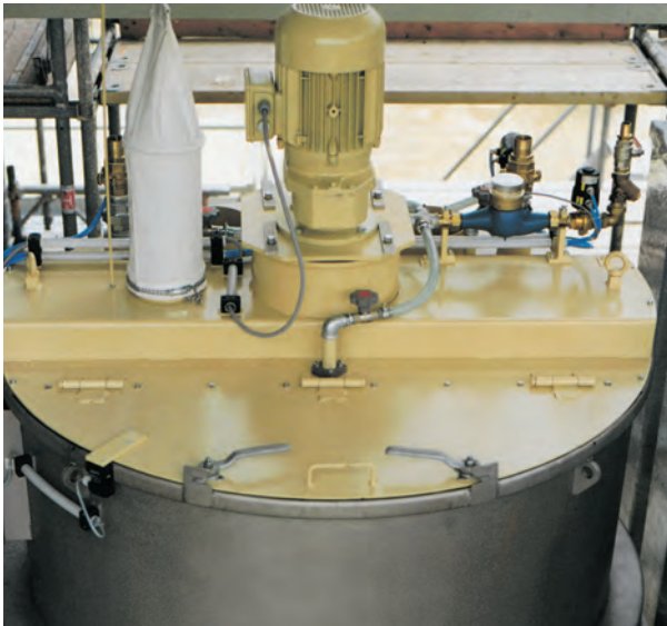
▲ Weighing and Mixing Station AHM 2020 capacity 2000 l, mixing tank on 3 load cells, for weighing different components, e.g. anhydrite, water, additives
