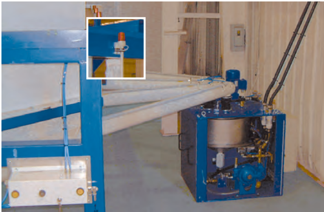
▲ Dry/Wet Metering System TFW 90 for 4 colors
