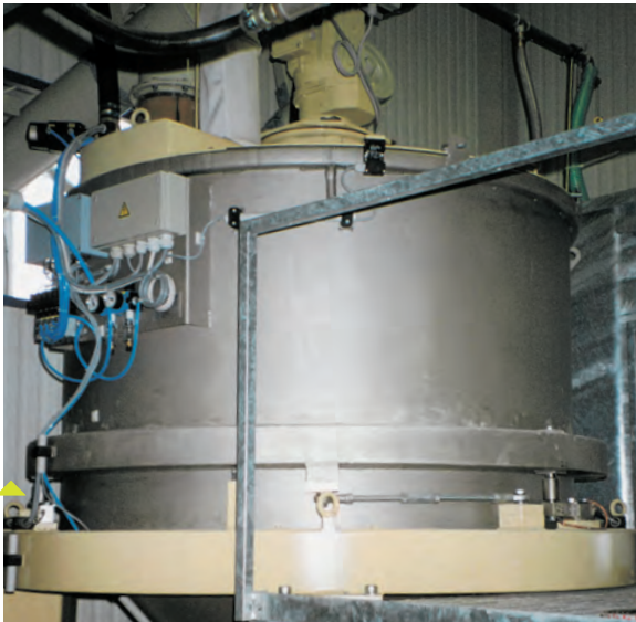
▲ Weighing and Mixing Station AHM 2020 capacity 2000 l, mixing tank on 3 load cells, for weighing different components, e.g. anhydrite, water, additives
