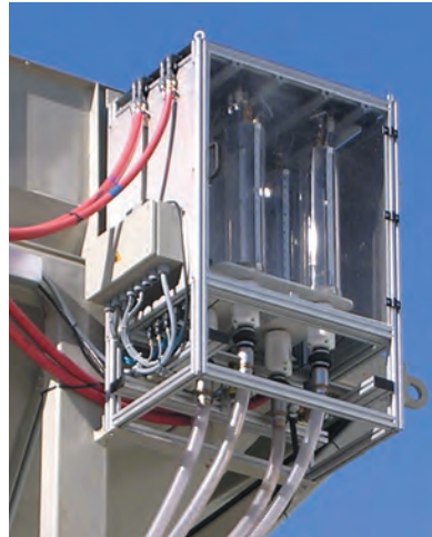
AC 5/5/15/15 weigher in protective cabinet, gravity discharge for 8 additives in 4 cylinders
