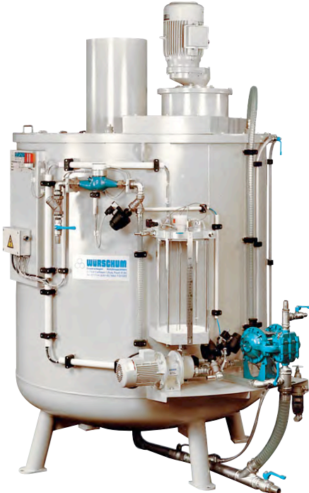
Mixing Tank MDI 3000 capacity 3000 l, with inlet for Big-Bag filling, and metering cylinder for additional chemical additive
