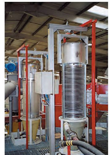
▲ CF 40-S filter cyclone with electronic load cell and easy to clean filter element
