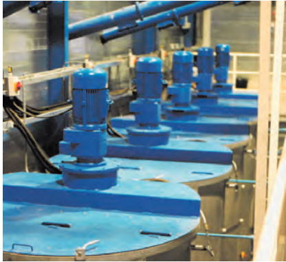
Mixing Tank MDI 8000 capacity 8000 l for iron oxide color slurry
