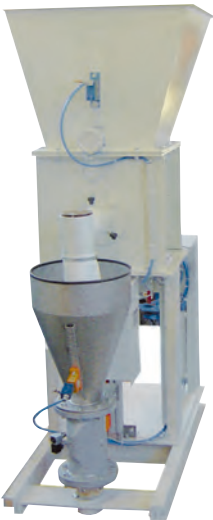
▲ Weigher PW 25, screw conveyors MD 100, hopper sizes 200 l
