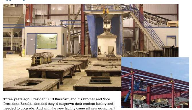
too. They hired ACT to install a Wiggert MobilMat MO80 - MO45 - 5 - PCS twin mixing/batching plant. Aside from allowing stripping, set-up functions, and casting (both dry-cast and wet-cast) to take place simultaneously for production flexibility, the ACT plant also features state-of-the-art data gathering. Everything from recording the production of every batch, to self-learning "in flight" correction capabilities provide all the automation and information they need.
