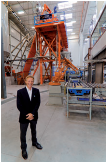
Charles Ciccarello, founder and president of Techo-Bloc, stands on the manufacturing floor of the new 80,000 sq. ft. Stonedge wet cast products plant his company recently completed in Chambly, Quebec, Canada. Just behind him is the Automacad-provided wet line (nearest) and (in orange in background) the ACT MobilMat mo2250-750 automatic concrete batching system.
