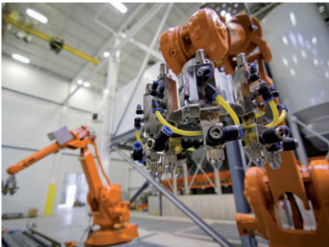
Automacad Color-I color application robots can deliver up to 14 colors for unlimited coloration patterns and non-repetitive effects. The robots apply color to the inside of the mold cavity, just prior to volumetric filling.
