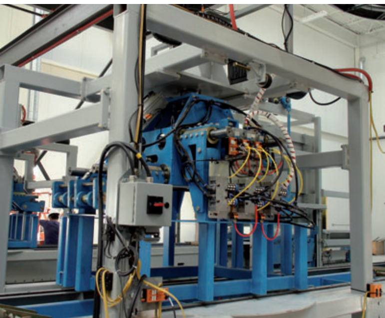
Automacad squeezer clamp is electrically and pneumatically powered and can handle blocks of nearly any design, size or height, prelocating them safely and easily in preparation for the packaging robot.
