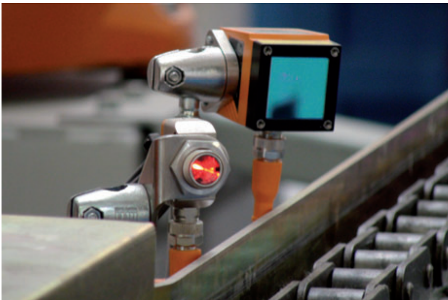
Automacad deployed sensors from ifm efector North America throughout the Stonedge plant to track product as it moves through the facility and feed information to the Automacad-designed SCADA central control system.
