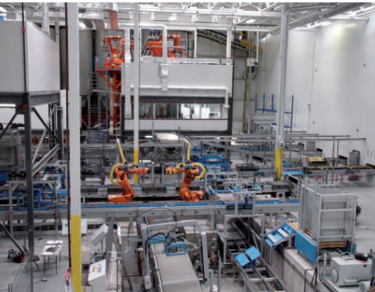
Dual Automacac product handling robots stand ready on the packaging lines in the foreground of this interior view of the new Stonedge wet cast concrete products facility outside of Montreal, Canada. Automacac, a Canadian design and manufacturing firm, engineered and produced more than 200 pieces of equipment for the new plant.
