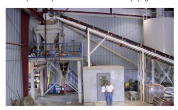
This MobilMat Mo45-2-PCS fully automatic turnkey concrete mixing batching plant from Advanced Concrete Technologies was installed in 2003 at Dalmaray Concrete Products in Janesville, Wisconsin. At left is the mixer platform, which includes a Wiggert HPGM 1125 high shear counter-current planetary mixer and at right a 50-ton cement silo. Dalmaray owner and President Rob Ausen stands in front of the plant control room.
