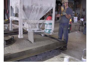
Dalmaray Precast casts most products using SCC (Self Consolidating Concrete) for better productivity and superior product quality. The SCC mix is delivered by crane bucket and provides consistent quality without vibration.
