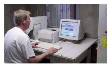
Dalmaray owner and President Rob Ausen uses the ACT Programmable Control System (PCS) to select recipes, track inventory, and monitor system functions. The PC-based system uses a graphical user interface (GUI) for intuitive control.
