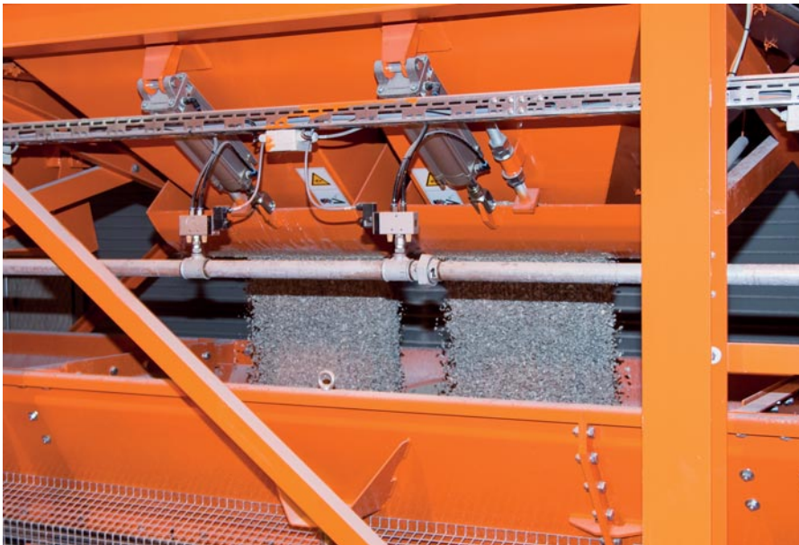
Each of three aggregate bins are equipped with dual batching gates for fast/slow precision batching performance.
