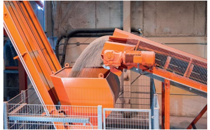
Skip hoists, loaded by transfer conveyor, are used to deliver aggregates to each of the ACT/Wiggert HPGM 2250 countercurrent mixers. At right is a three-compartment aggregate storage bin with weight belt below and at left is one of two mixer platforms.
