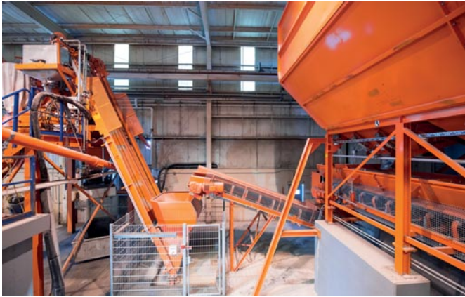
Skip hoists, loaded by transfer conveyor, are used to deliver aggregates to each of the ACT/Wiggert HPGM 2250 countercurrent mixers. At right is a three-compartment aggregate storage bin with weight belt below and at left is one of two mixer platforms.
