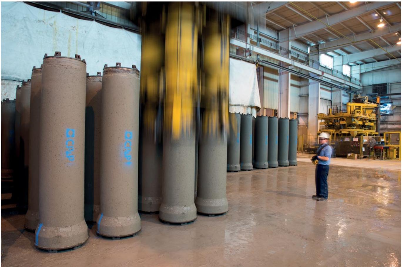
A four-pack of reinforced concrete pipes, produced on a HawkeyePedershaab PipePro XT production system, are demolded in the curing area at the CP&P Jessup facility. The plant produces an average of 500 tons of precast pipe daily.
