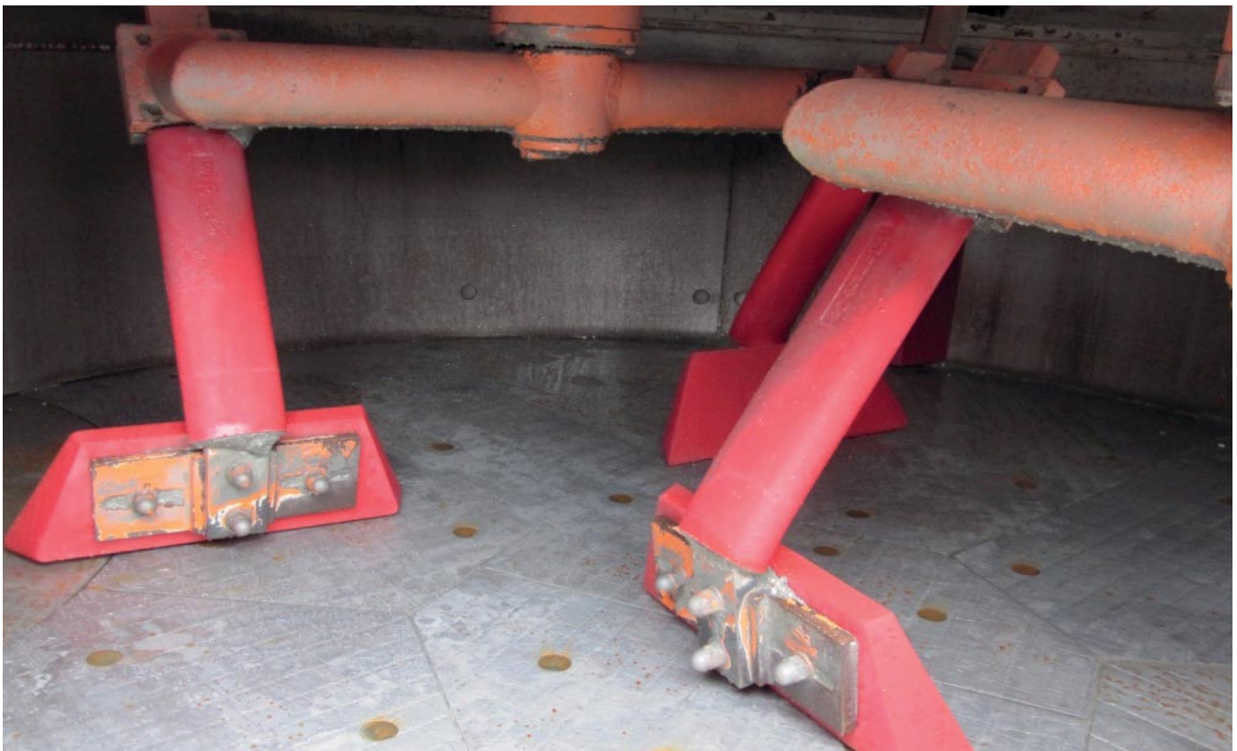
Interior HPGM mixer features long-wear replaceable plating and countercurrent high shear mixing tools.
